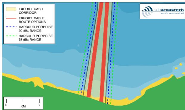
Figure 5-1 Contour plot showing the 90 and 75 dB<sub>re</sub> impact ranges for harbour porpoise during trenching operations
